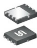
TSM160P04LCRHLG TSC (Taiwan Semiconductor) MOSFET P-CH 40V 51A 8PDFN
