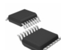
ADF4154BRUZ Analog Devices Inc. IC FRAC-N FREQ SYNTH 16- TSSOP
