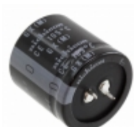
LGX2G471MELC35 Nichicon CAP ALUM 470UF 20% 400V SNAP
