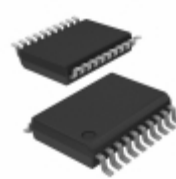
PIC16F716T-I/SS Microchip Technology IC MCU 8BIT 3.5KB FLASH 20SSOP
