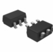
MIC5321-SLYD6-TR Microchip Technology IC REG LDO 3.3V/2.7V TSOT23-6
