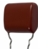
ECQ-P1H334GZW Panasonic Electronic Components CAP FILM 0.33UF 2% 50VDC RADIAL
