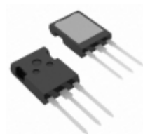
IXFX21N100F IXYS RF MOSFET N-CH 1000V 21A PLUS247-3
