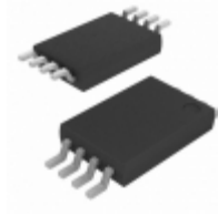
IRF7705 International Rectifier (Infineon Technologies) MOSFET P-CH 30V 8A 8-TSSOP
