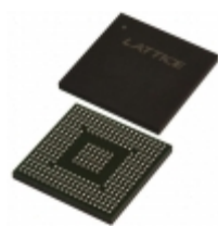
LCMXO2-7000HE-5BG332I Lattice Semiconductor Corporation IC FPGA 278 I/O 332CABGA
