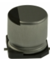
EEE-HAA102UAP Panasonic Electronic Components CAP ALUM 1000UF 20% 10V SMD
