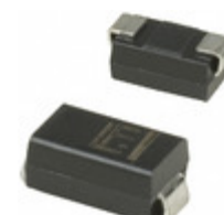
P4SMA43C Littelfuse Inc. TVS DIODE 36.8VWM 62.27VC SMD
