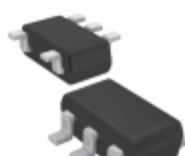
XC6123C743MR-G Torex Semiconductor Ltd IC WATCHDOG TIMER SOT-25
