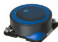
SLF10145T-152MR22-H TDK Corporation FIXED IND 1.5MH 260MA 3.4 OHM
