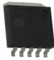
MIC37152WR Microchip Technology IC REG LDO ADJ 1.5A SPAK-5
