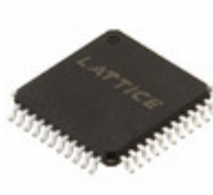
ISPLSI 1016E-80LT44I Lattice Semiconductor Corporation IC CPLD 64MC 15NS 44TQFP
