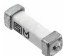
3405.0175.24 Schurter Inc. FUSE BOARD MNT 8A 250VAC 125VDC
