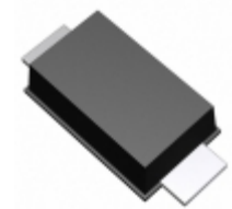
KDZTR8.2B LAPIS Semiconductor DIODE ZENER 8.7V 1W PMDU
