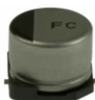
EEE-FC1V470AP Panasonic Electronic Components CAP ALUM 47UF 20% 35V SMD
