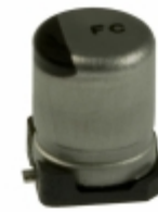
EEE-FC1V2R2R Panasonic Electronic Components CAP ALUM 2.2UF 20% 35V SMD
