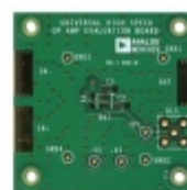
AD8009JRT-EBZ ADI (Analog Devices, Inc.) BOARD EVAL FOR AD8009
