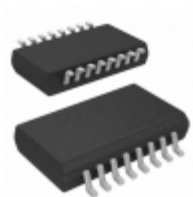
ADUM152N1BRZ-RL7 Analog Devices Inc. DGTL ISO 3KV GEN PURP 16SOIC
