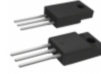
BYVF32-100HE3/45 Electro-Films (EFI) / Vishay DIODE ARRAY GP 100V 18A ITO220AB
