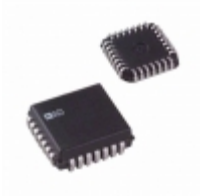
AD7547KP Analog Devices Inc. IC DAC 12BIT DUAL LC2MOS 28-PLCC
