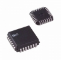
AD7547JPZ-REEL Analog Devices Inc. IC DAC 12BIT DUAL LC2MOS 28-PLCC
