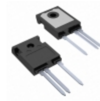
IXTH1N170DHV IXYS Corporation MOSFET N-CH
