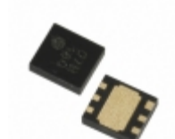
XC6124E520ER-G Torex Semiconductor Ltd IC WATCHDOG TIMER 6-USP
