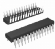
PIC24HJ128GP202-I/SP Microchip Technology IC MCU 16BIT 128KB FLASH 28SDIP
