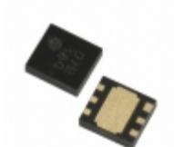
XC6122F650ER-G Torex Semiconductor Ltd IC WATCHDOG TIMER 6-USP
