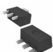
AP7365-20YG-13 Diodes Incorporated IC REG LDO 2V 0.6A SOT-893L
