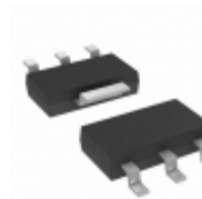
AP7365-20ERG-13 Diodes Incorporated IC REG LDO 2V 0.6A SOT-2233L
