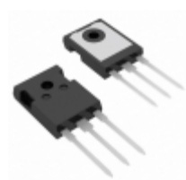
IXXH60N65B4 IXYS IGBT 650V 116A 455W TO247AD
