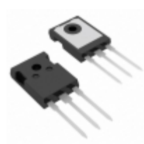
IXXH50N60B3D1 IXYS IGBT 600V 120A 600W TO247
