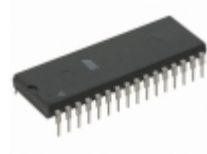
AT49LV002T-12PC Microchip Technology IC FLASH 2MBIT 120NS 32DIP
