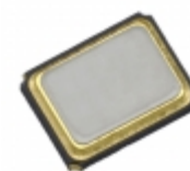
FA-128 50.000MD50X-G3 EPSON CRYSTAL 50.00 MHZ 20.0PF SMD
