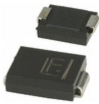
SMCJ40C Littelfuse Inc. TVS DIODE 40VWM 67.73VC SMC
