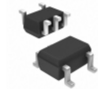
74LVCE1G08SE-7 Diodes Incorporated IC GATE AND 1CH 2-INP SOT-353
