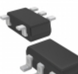
XC6124C422MR-G Torex Semiconductor Ltd IC WATCHDOG TIMER SOT-25
