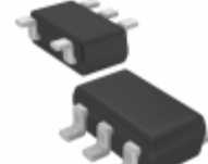
XC6124C425MR-G Torex Semiconductor Ltd IC WATCHDOG TIMER SOT-25
