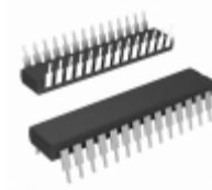
PIC24FJ32MC102-I/SP Microchip Technology IC MCU 16BIT 32KB FLASH 28SDIP
