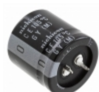
LGY2A152MELB30 Nichicon CAP ALUM 1500UF 20% 100V SNAP
