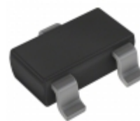
BCW72T116 Rohm Semiconductor TRANS NPN 45V 0.1A SST3
