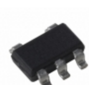
MIC5207-2.9YM5-TR Microchip Technology IC REG LDO 2.9V 0.18A SOT23-5
