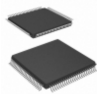
CY7C09189V-6AXC Cypress Semiconductor Corp IC SRAM 576KBIT 6.5NS 100TQFP
