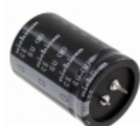
LGU1E333MELC Nichicon CAP ALUM 33000UF 20% 25V SNAP
