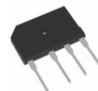
TS25P03GHC2G TSC (Taiwan Semiconductor) BRIDGE RECT 1P 200V 25A TS-6P
