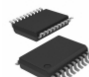
PIC18F14K50-I/SS Microchip Technology IC MCU 8BIT 16KB FLASH 20SSOP
