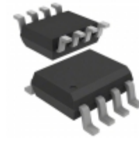
ADM706TARZ-REEL Analog Devices Inc. IC SUPERVISOR MPU 3.08V WD 8SOIC
