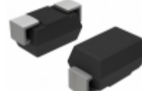
SMAJ110CA Bourns Inc. TVS DIODE 110VWMM 177VC DO214AC
