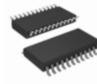
ICL3207CBZ Intersil IC 5DRVR/3RCVR RS232 3V 24-SOIC
