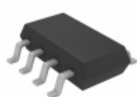
LTC2632CTS8-LI12#TRMPBF Linear Technology IC DAC 12BIT SPI/SRL TSOT-23-8
