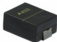
CU4032K50G2 EPCOS (TDK) VARISTOR 82V 1.2KA 4032
