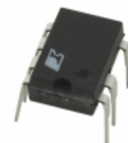
TOP258PN Power Integrations IC OFFLINE SWIT PROG OVP 8DIP
