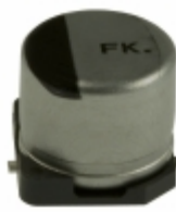
EEE-FKE101XAP Panasonic Electronic Components CAP ALUM 100UF 20% 25V SMD
