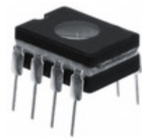
PIC12CE674/JW Microchip Technology IC MCU 8BIT 3.5KB EPROM 8CDIP
