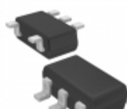
XC6123D642MR-G Torex Semiconductor Ltd IC WATCHDOG TIMER SOT-25
